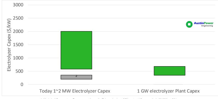
1. Made in US or western Europe countries; cell efficiency is about 85%; output H2 gas purity is 99.99% at 30 barg 2. Units made in China and sold in China only; as low as \$200~300/KW
