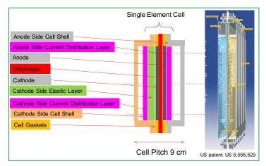
Future Alkaline Scenario: 10 MW Atm. Pressure Alkaline Electrolyzer Stack
