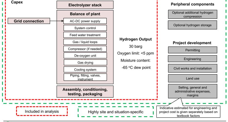
Comparing large scale hydrogen electrolysis plant with small hydrogen electrolyzer, cost reduction mainly comes from the following areas:
